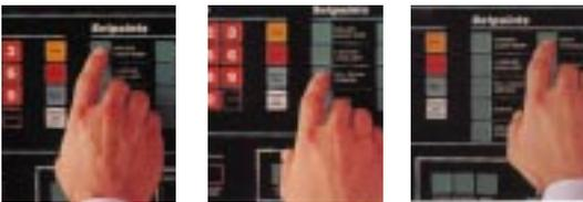
control and monitoring functions. Keys are clearly labeled and amply spaced to avoid “neighbor-key” errors, and each key is dedicated to one function, eliminating confusion.
